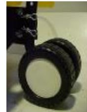
Then fit the depth skid and wheel clamp using the two cotter bolts supplied.
